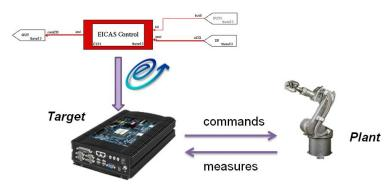
This demo shows all the main features connected to the Target operative mode: Automatic Code Generation for target, Hardware-in-the-loop and Final Validation Test. The following diagrams show respectively the roles of the element of the scenario in the two operative sub-modes respectively.
